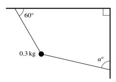
A particle of mass  $0.3\,\mathrm{kg}$  is held at rest by two light inextensible strings. One string is attached at an angle of  $60^\circ$  to a horizontal ceiling. The other string is attached at an angle  $\alpha^\circ$  to a vertical wall (see diagram). The tension in the string attached to the ceiling is  $4\,\mathrm{N}$ .
