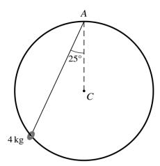
A ring of mass  $4 \, \text{kg}$  is threaded on a smooth circular rigid wire with centre C. The wire is fixed in a vertical plane and the ring is kept at rest by a light string connected to A, the highest point of the circle. The string makes an angle of  $25^{\circ}$  to the vertical (see diagram).
