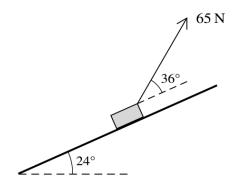
A block of mass 12 kg is placed on a plane which is inclined at an angle of 24° to the horizontal. A light string, making an angle of 36° above a line of greatest slope, is attached to the block. The tension in the string is 65 N (see diagram). The coefficient of friction between the block and plane is  $\mu$ . The block is in limiting equilibrium and is on the point of sliding up the plane.
