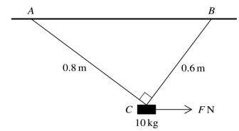
The diagram shows a block of mass  $10\,\mathrm{kg}$  suspended below a horizontal ceiling by two strings AC and BC, of lengths  $0.8\,\mathrm{m}$  and  $0.6\,\mathrm{m}$  respectively, attached to fixed points on the ceiling. Angle  $ACB = 90^\circ$ . There is a horizontal force of magnitude FN acting on the block. The block is in equilibrium.
