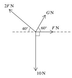
Four coplanar forces act at a point. The magnitudes of the forces are  $10\,\mathrm{N}$ ,  $F\,\mathrm{N}$ ,  $G\,\mathrm{N}$  and  $2F\,\mathrm{N}$ . The directions of the forces are as shown in the diagram.
