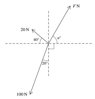
Three coplanar forces of magnitudes  $20\,\mathrm{N}$ ,  $100\,\mathrm{N}$  and  $F\,\mathrm{N}$  act at a point. The directions of these forces are shown in the diagram.
