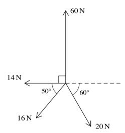
Coplanar forces of magnitudes  $60\,N$ ,  $20\,N$ ,  $16\,N$  and  $14\,N$  act at a point in the directions shown in the diagram.
