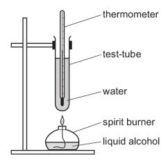
Describe how the apparatus shown can be used to compare the amount of energy given out by three different liquid alcohols, ethanol, propanol and butanol. Your answer should include how the results can be used to determine which fuel gives out the most energy.
