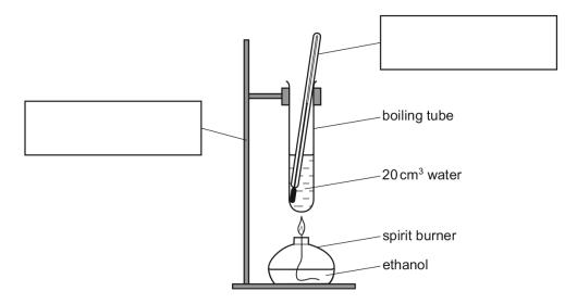
The ethanol was burned for one minute. The temperature of the water was then measured and recorded.
