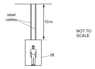
The cables extend by 1 mm when a man of mass 80 kg steps into the lift.
